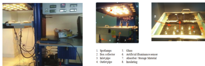
FIGURE 1. Solar thermal energy unit
